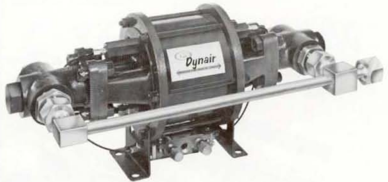
Air-Operated Booster Pump . . . DYNAIR™ double acting pump delivers up to 5,000 or 10,000 psi with an air supply pressure of 80 to 100 psi.
