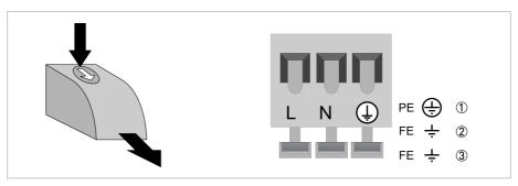
Figure 4-5: Power supply connection
