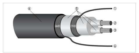
Figure 4-1: Construction of signal cable A
