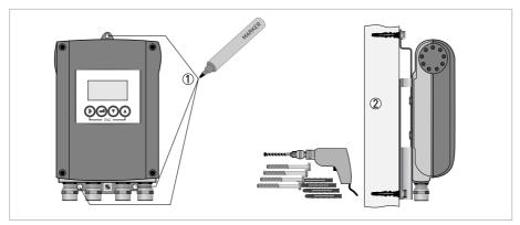
Figure 3-1: Mounting the wall-mounted housing
